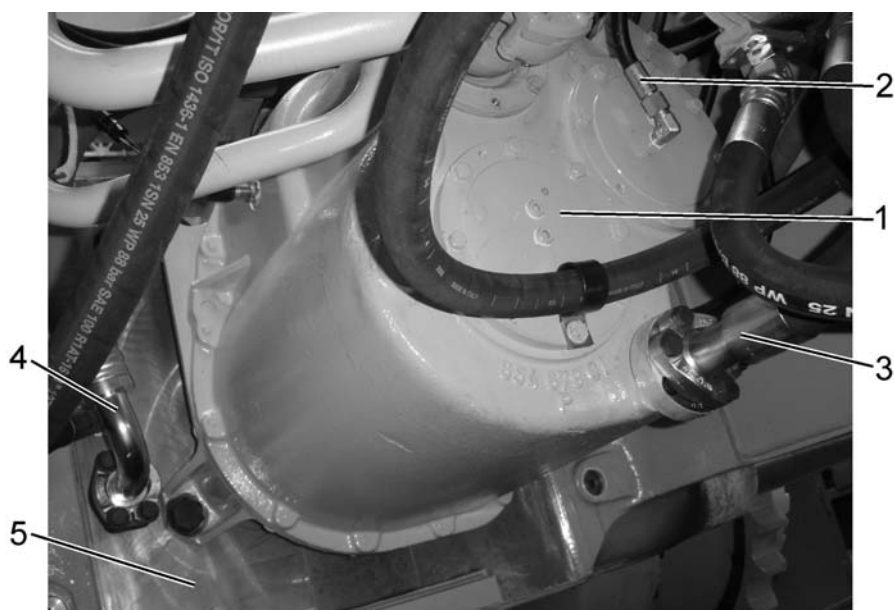
Fig. 7C.3. Transmission Disconnecting Points (Bottom View)
