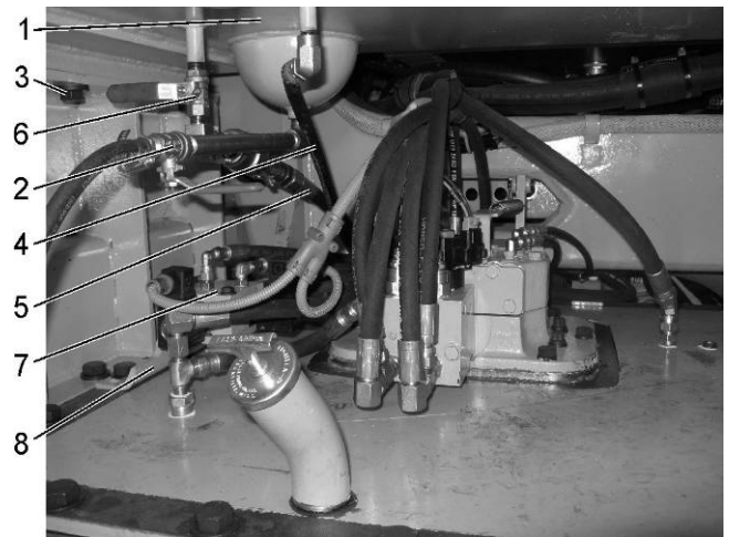
Fig. 7E.2. Fuel Line Disconnecting Points
