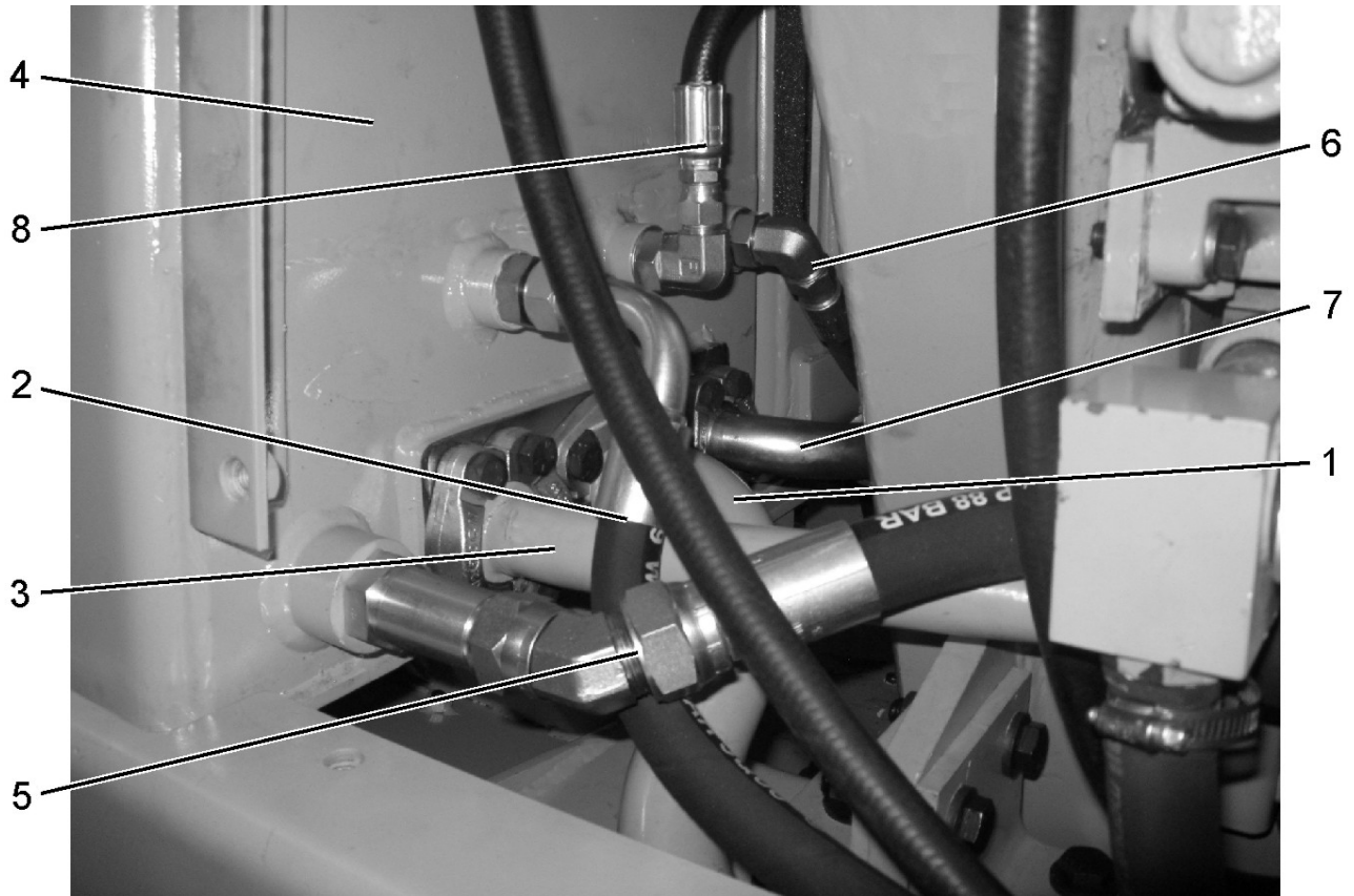
Fig. 10E.3. Hydraulic Reservoir Disconnecting Points
