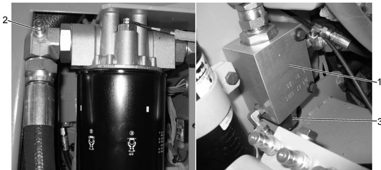
Fig. 7.11. Priority Valve Pressure Gauge Connect Point
