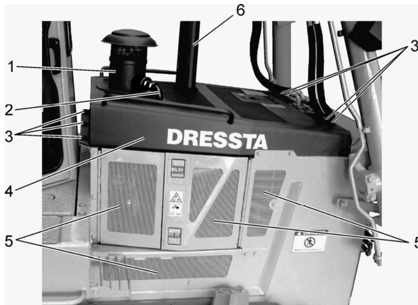
Fig. 6.2. Hood and Engine Enclosure
