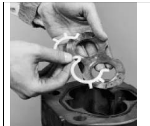
S – Flat Side of Seal Assy W – Wear Plate
