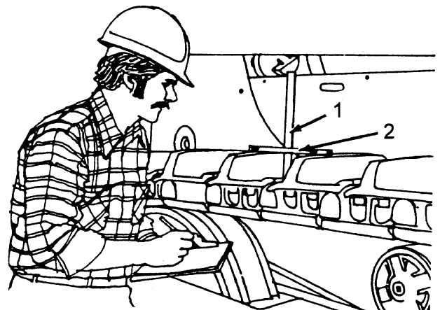
Fig. 14.4. Measuring Grouser Height
