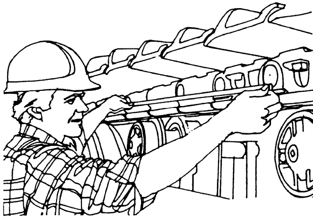
Fig. 14.7. Measuring Track Pitch
