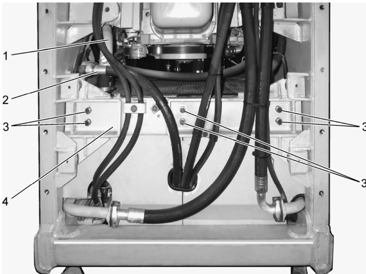
Fig. 6.6. Radiator Assy Disassembly Points (bottom view)
